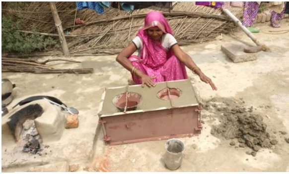
Making smokeless chulha through mould and usage of chulha by women from the dolphin village
